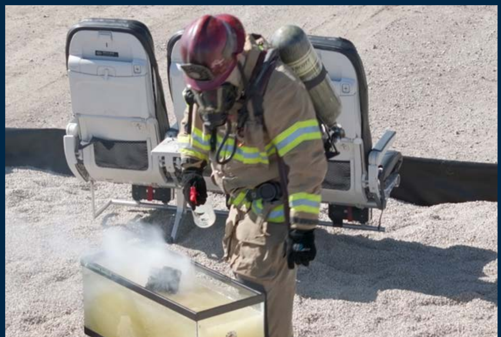
Burning laptop - Lithium-Ion battery with thermal runaway on airline simulation demo
