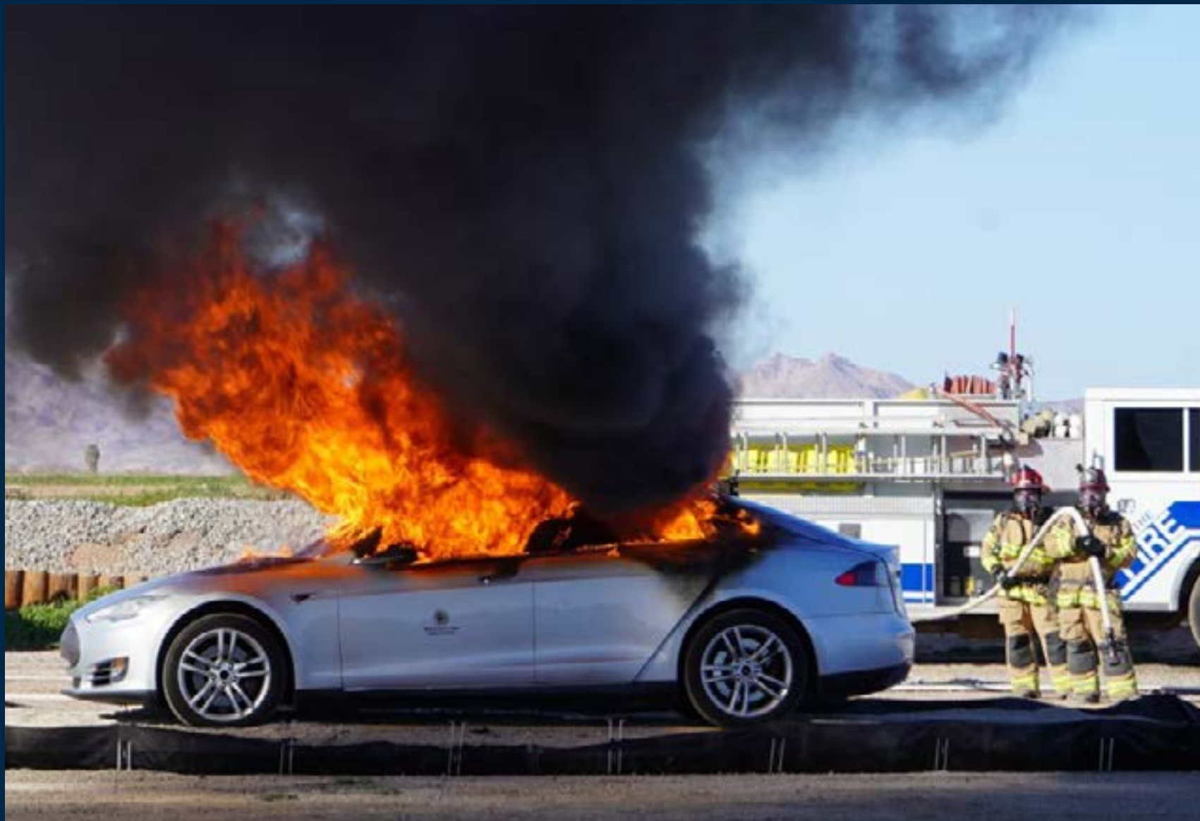
Lithium-ion battery fire in EV during product testing by SFS team members in Blythe, CA
