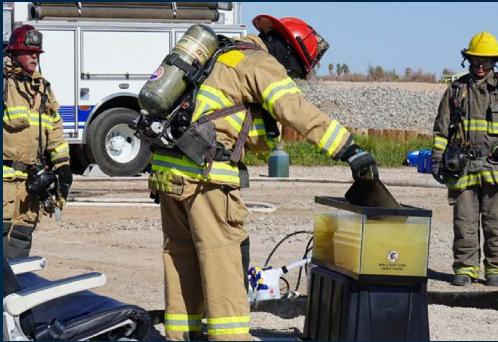
Burning laptop - Lithium-Ion battery with thermal runaway submerged during product testing
